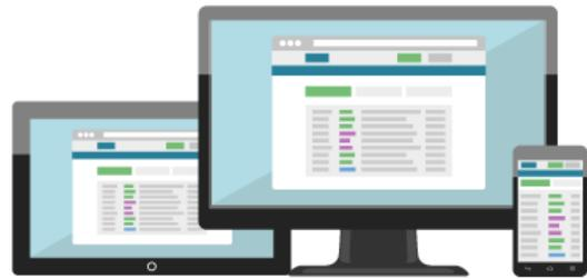
Any number of recipients can receive notifications based on Fire Alarm event types: Fire, Pre Fire, Fault, Isolation, Disablement etc. Each event notification details the event action, the associated control panel descriptive labels and protocol data. Notifications are triggered and processed immediately.
